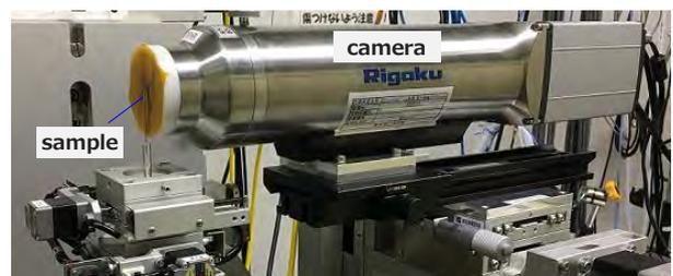
Fig. 1. X-ray CT measurement setup.
