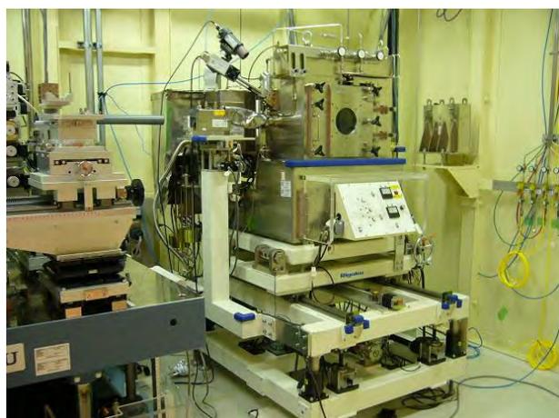
Fig. 1. X-ray fluorescence analyzer at BL16XU.
