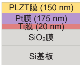
Fig. 2. Schematic drawing of the deposited layer sequence.
