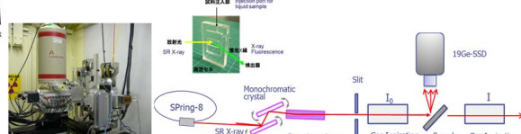
Fig.2 XAFS measurement apparatus and liquid sample holder
