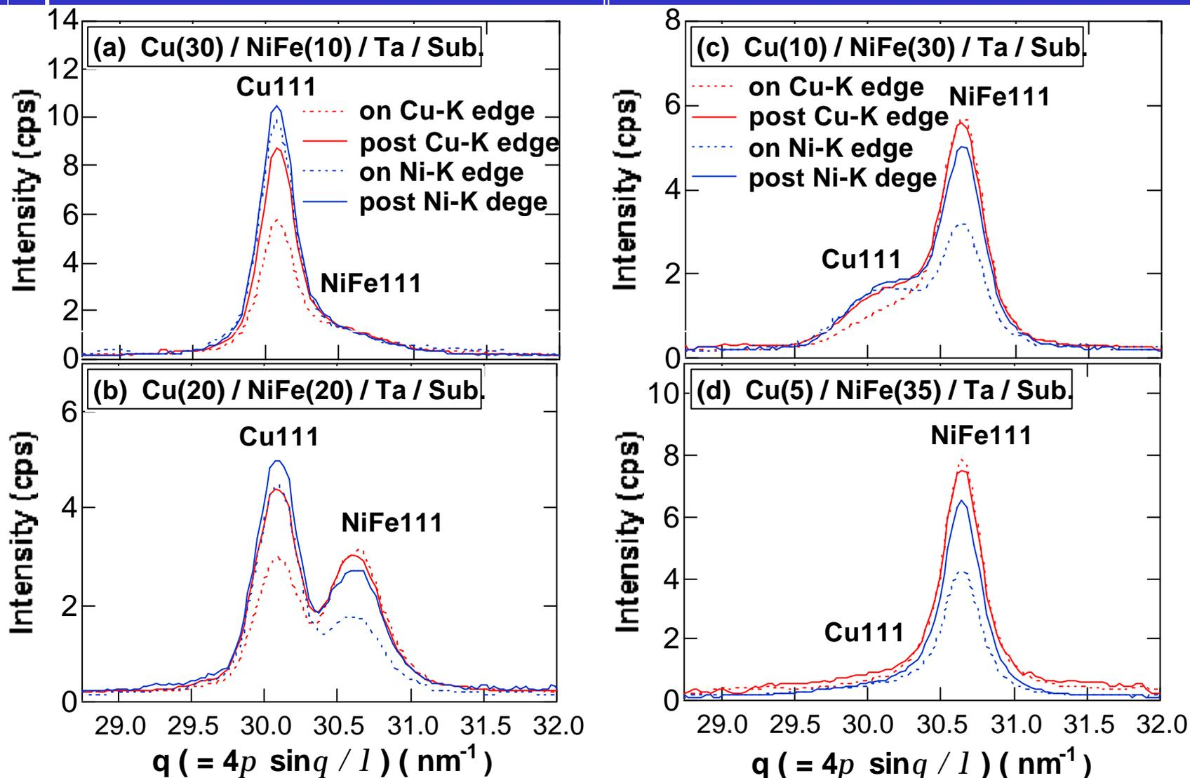
**Fig.4 111 Diffraction patterns for the samples to stack Cu and NiFe measured at four wavelengths.**
