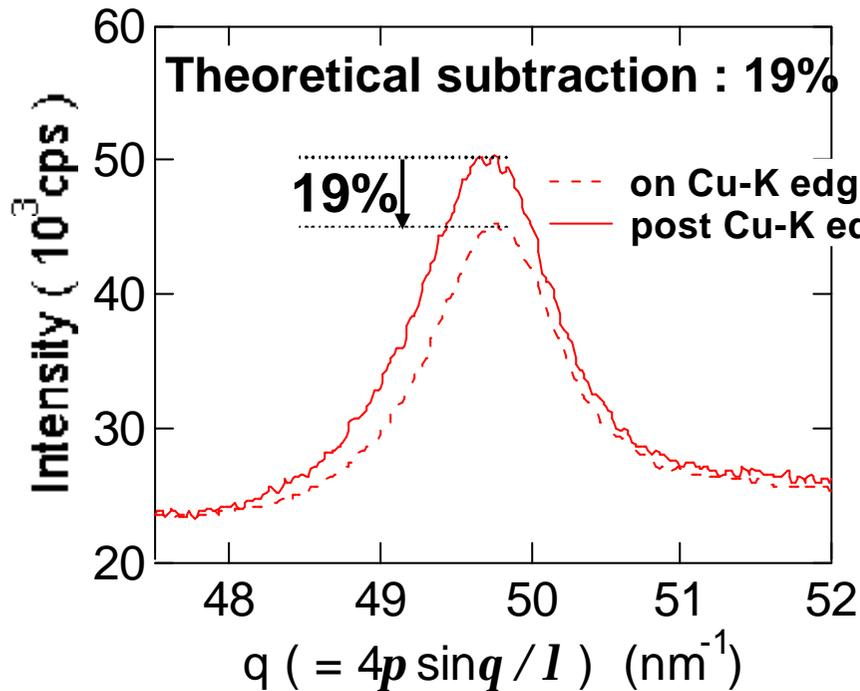
(a) Differential Cu diffraction patterns at near Cu-K edge.
