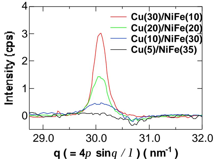
(a) Differential Cu diffraction patterns at near Cu-K edge.
