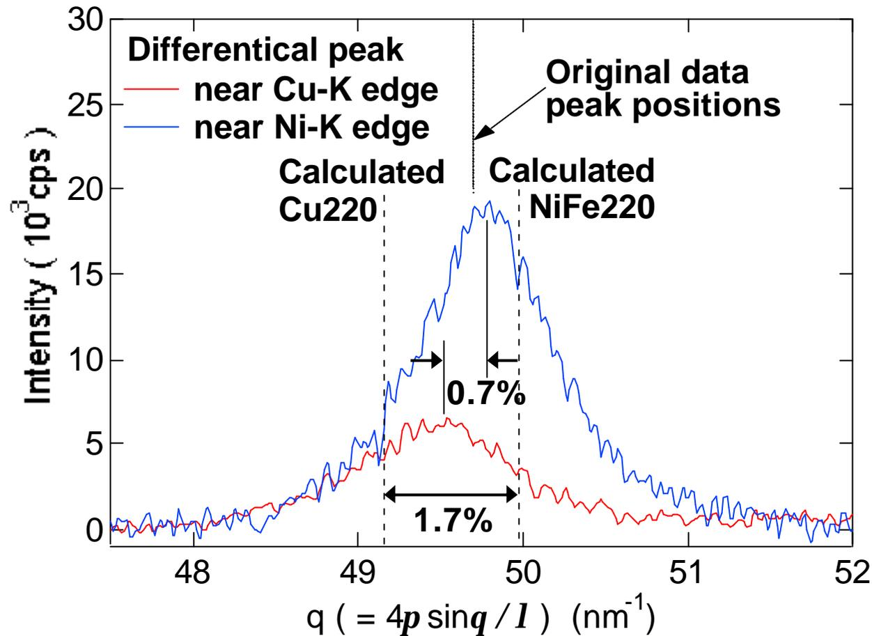
**Fig.9 Differential Cu and NiFe diffraction patterns.**
