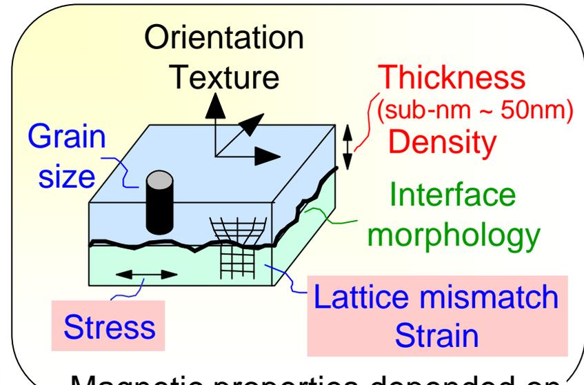
Magnetic properties depended on structure of the magnetic layers
