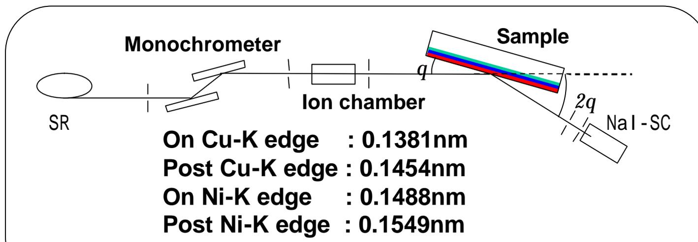
Fig.2 Schematic of x-ray optics for a symmetry diffraction
