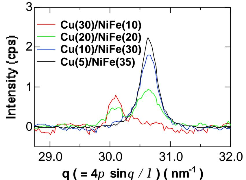
(b) Differential NiFe diffraction patterns at near Ni-K edge.
