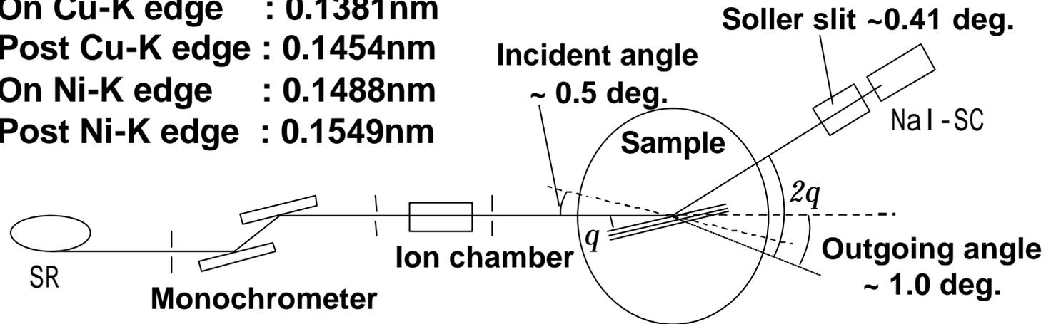
**Fig.8 Schematic of x-ray optics for a in-plane diffraction**
