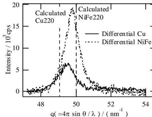
Fig.1 Differential Cu and NiFe diffraction patterns (post edge – K-edge pattern). Two dashed lines show the peak positions based on JCPD.
