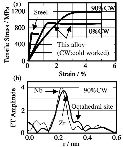
Fig.1: Mechanical properties (a) and Fourier transformed spectra (b) of this alloy.
