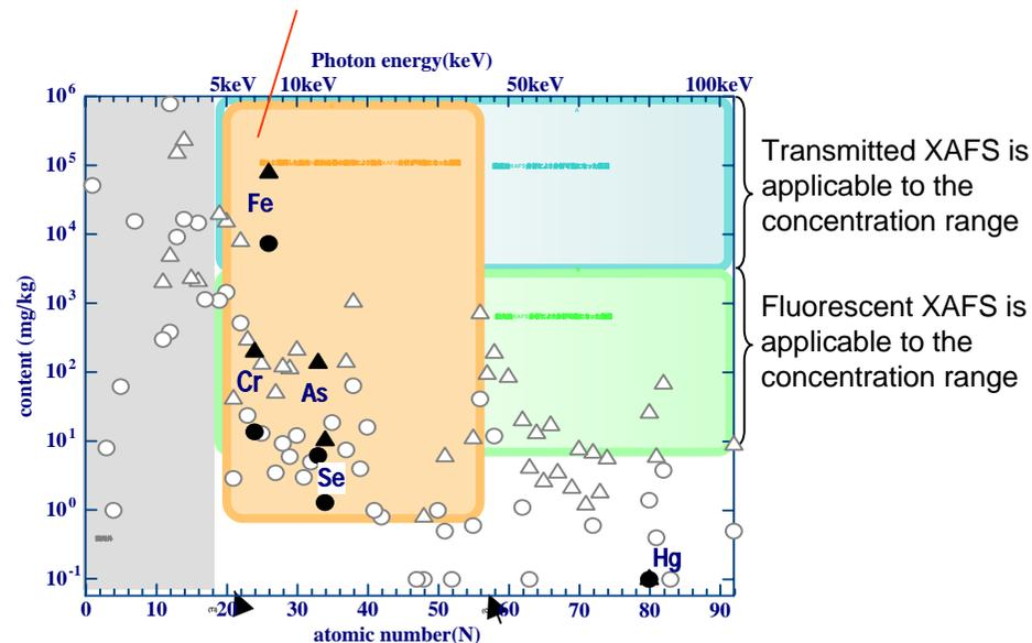
**Figure 6.** Capability of XAFS analysis on the speciation of various elements in typical bituminous coal and fly ash.
