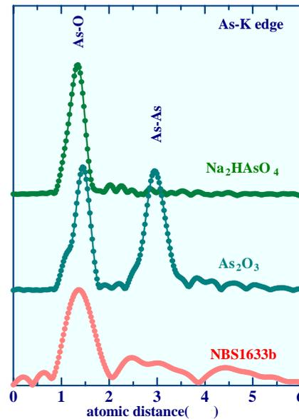
Figure 3. EXAFS spectra of arsenic contained in fly ash specimens.
