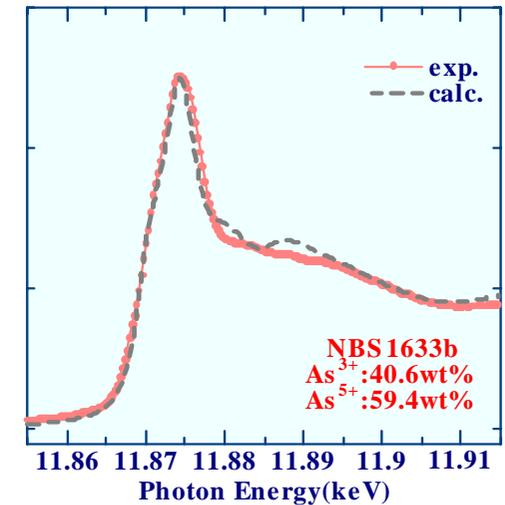
**Figure 2.** XANES spectra of arsenic contained in coal and fly ash and their curve fits assuming chemical form of the components.
