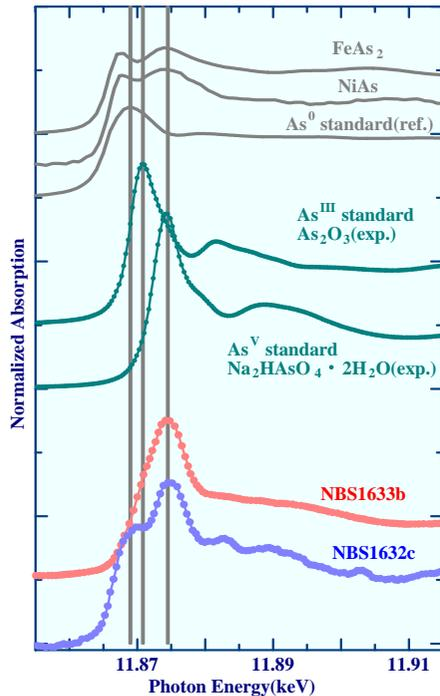
**Figure 1.** XANES spectra of arsenic contained in coal and fly ash.
