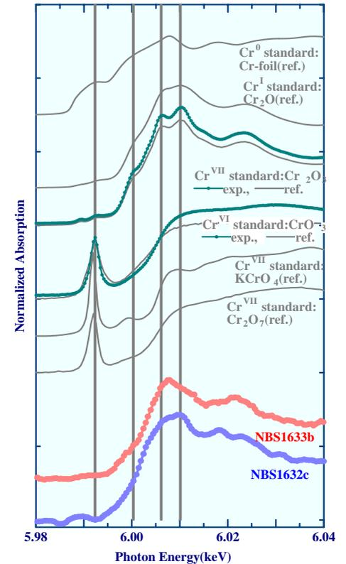
Figure 4. XANES spectra of chromium contained in the specimens.
